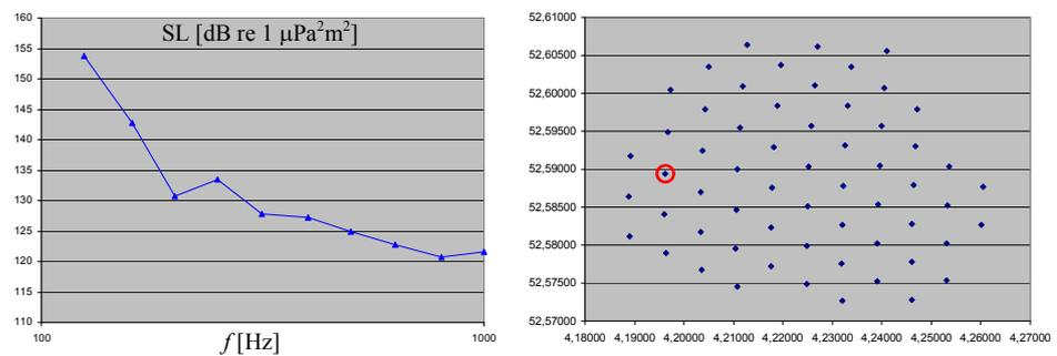
Figure 6.12. 1/3-octave source level spectrum of wind turbine *Paludans Flak* (left) and (proposed) locations (decimal lon-lat) of wind turbines in the Q7 wind farm (right; red circle marks monopile #42).
