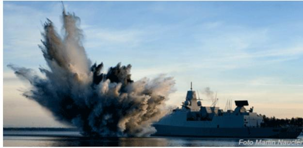
Figure 4.10. Shock testing of the air-defence and command frigate Hr.Ms. Evertsen at the Stockholm Archipelago.
