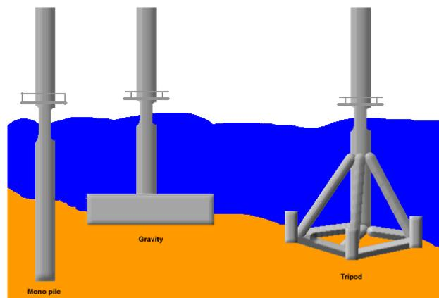
Figure 4.12. Overview of basic offshore wind turbine foundation types (source: [offshorewind.net/Other\\_Pages/Turbine-Foundations](http://offshorewind.net/Other_Pages/Turbine-Foundations)).
